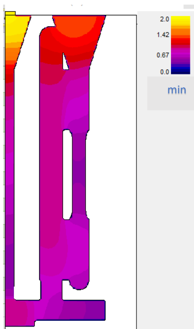
Figure 8. Modeled distribution of the solidification time.
